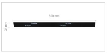
This type of panel is approx. 34 mm thick excluding the top layer that must still be applied.
