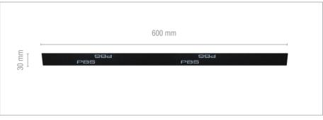
This type of panel is approx. 30 mm thick not including the top layer to be applied afterwards.
