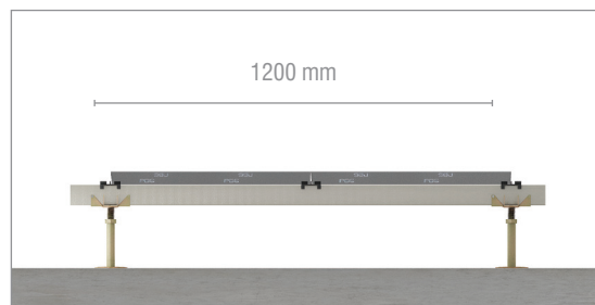
The grid size of this substructure is 600 mm x 1,200 mm. Different sizes are possible.
